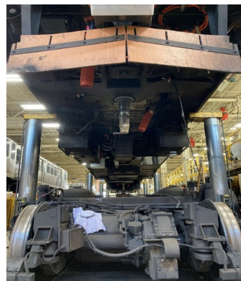
CTA's 5000-Series rail car has old truck removed from married pair.
